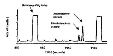
As shown in this figure, the chromatogram has clean, well-defined peaks, that are well-separated. Figure taken from: R. Aguilera *et al.*, Rapid Commun. Mass Spectrom., 14 2294, 2299 (2000).
