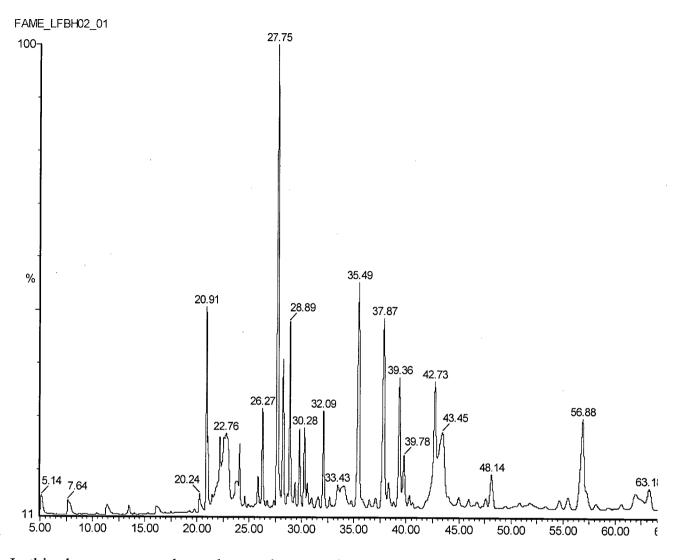
In this chromatogram, the peaks are close together, overlapping and not well-defined. The consequences for the final delta C13 vales are tremendous, often resulting in sharply varying values for target analytes.
